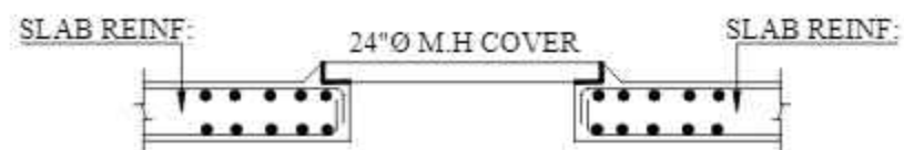
REINFORCEMENT DETAIL OF MAIN HOLE TYP.
